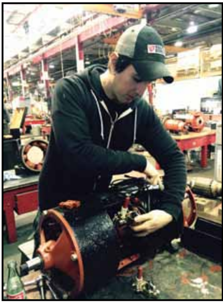
Darren Hawe, a 32-year-old second class electrical worker at the Everett shop with Local 717 IBEW, repairs a 129MG generator used in the Mattapan fleet of PCC cars. BillForryphoto
