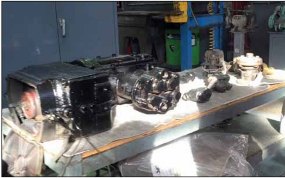
This original Westinghouse DH10 air compressor — a vital component of the PCC cars used on the Mattapan Line — is shown at a work station inside the MBTA's Everett Shops. This "genius" piece of equipment powers a range of equipment in the trolley, from doors and brakes to windshield wipers.
