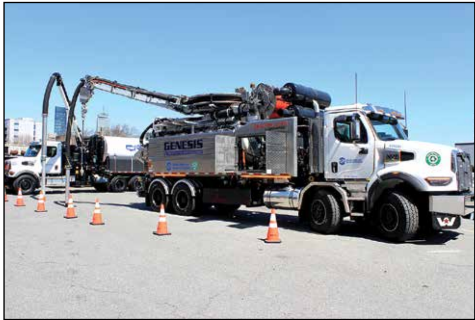
The Genesis, a specialized truck acquired by the Boston Water and Sewer Commission, will help clean the city’s sewer and storm drains while saving water and money, according to agency officials. At right: Part of the BWSC’s new fleet of electric vehicles get charged up at a Roxbury garage.
