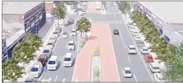
This rendering gives a rough idea of one of three concepts being shopped around the community right now for Mattapan Square. While this rendering includes adding a bus lane and switching to parallel parking, others consist of having no center bus lane and keeping angled parking (existing conditions), or adding a center bus lane and keeping angled parking. The BTD hopes to have a concept consensus formed by the end of the summer to be able to move on with a final design.
