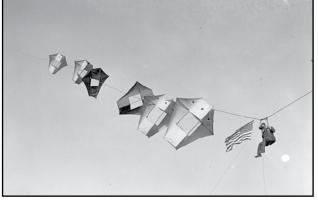
raise a man. A ground crew operating a winch could reel the "pilot" in or out depending on the weather, or what he needed to see.
