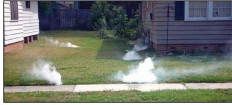
A Boston Water & Sewer image shows smoke tests in progress.
