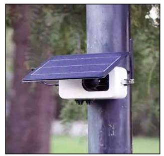
the technology for air quality sensors has improved rapidly, making high-quality sensing available in a "shoebox size" instrument that runs on solar power with a battery back-up.
